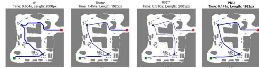
Fig. 14. Path comparison in construction site environment for four algorithms. (a) A*, (b) Theta*, (c) RRT*, (d) PNU.
